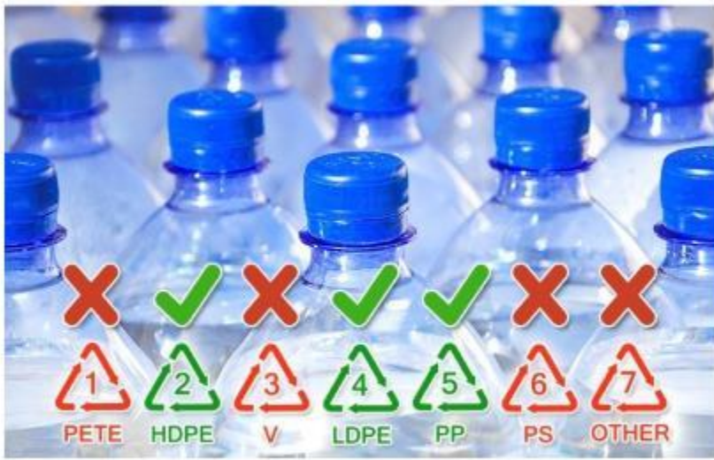
Bottles made of polyethylene (2 and 4) and polypropylene (5 and PP) are suitable for multiple uses . They're relatively safe if you only store cold water in them and regularly disinfect them.
